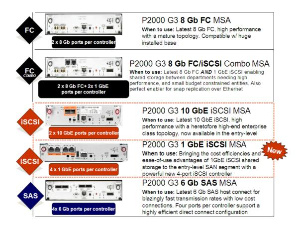
Capacity can easily be added as the need develops by attaching additional drive enclosures. Maximum capacity ranges with LFF drives up to 134 TB SAS or 288 TB SAS Midline or 192 TB SATA Midline with the addition of the maximum number of drive enclosures. Configurations utilizing the SFF drive chassis and the maximum number of drive enclosures can grow to 134 TB of SAS or 149 TB of SAS Midline or 74.5 TB SATA Midline with a total of 96 LFF or 149 SFF drives.
